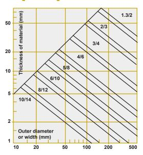
This diagram is a guide to help you chose the correct tooth pitch when cutting pipes and profiles. The very best choice is in the area where a line from the outer diameter crosses a line from the thickness of the material.
