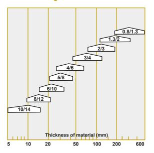
This diagram is a guide to help you chose the correct tooth pitch when cutting solid work pieces. The very best choice is where the tooth pitch-area is at its widest.
